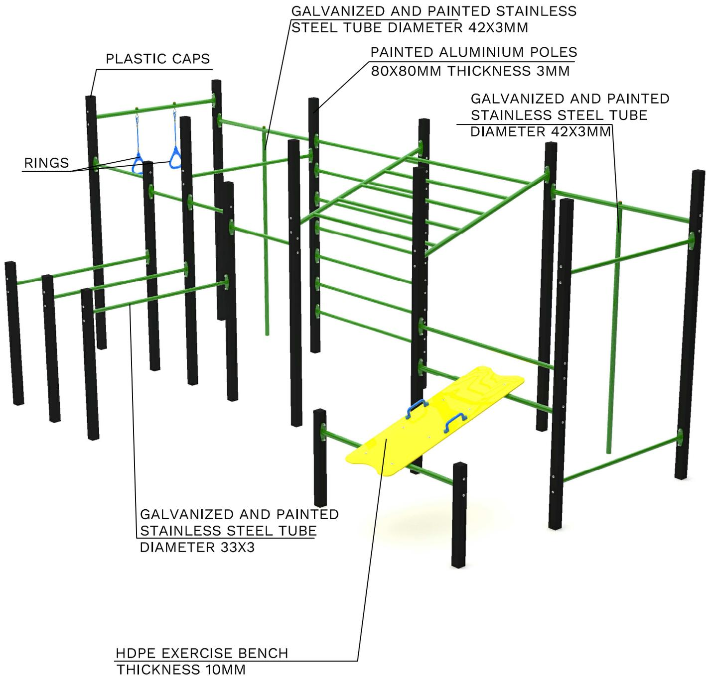
ALL THE FIXING ELEMENTS, SCREWS, DROWS, ECC .. ARE IN STAINLESS STEEL AND PROTECTED WITH PLASTIC BOLTS AND CAPS.
